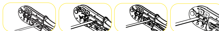
Strip CAT.5 cables Strip cables w/build-in stopper length Cut cables Build-in crimp modular for 8P/6P
