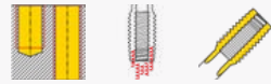
through holes & blind holes up to 1,5 x D Chip removal (like picture) Form C straight flutes
